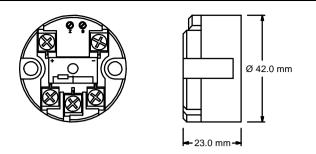
Mounting holes: 2 holes 5.5mm diameter, 33mm centres Centre hole sensor wire entry: 4.0mm diameter
