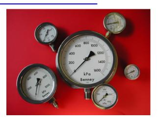
Note for all gauges: <u>DO NOT</u> under any circumstances remove the rubber diaphragm or plug from the top of the gauge. The gauge Breather Plug orientation must be in an upright position.
